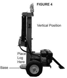
3. In FIGURE 1, the Rail Assembly (2) is shown in Horizontal mode for operation and travel. In FIGURE 4 the unit is shown in the vertical position. To change positions, remove the Hair Pin Clip (29) and the Push Pin (26). A close-up of this Push Pin is shown in FIGURE 3. Tilt the unit to the vertical position as shown in FIGURE 4, and replace both the Push Pin and the Hair Pin Clip into the vertical position hole (See FIGURE 1). Reverse the process to return to the horizontal position.
